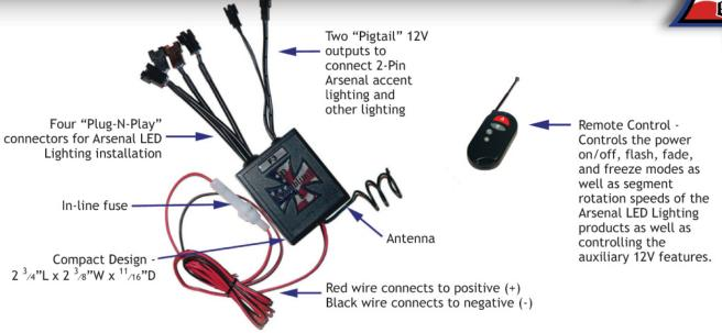
Rumbling Pride's Freedom Series Electronic Control Module (ECM) is the core of the Arsenal LED Lighting System. Feature rich, our ECM provides 100% remote controlled functionality that is unrivaled, and raises the bar when it comes to LED lighting effects.
